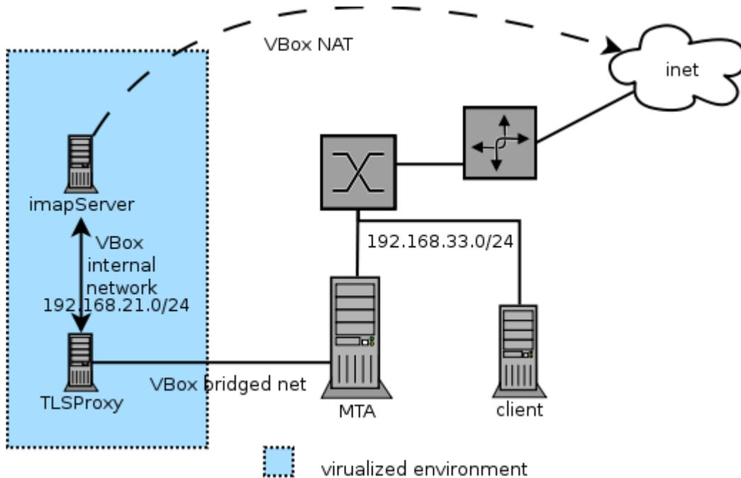
*Illustration 22: environment during long term test: network architecture*
