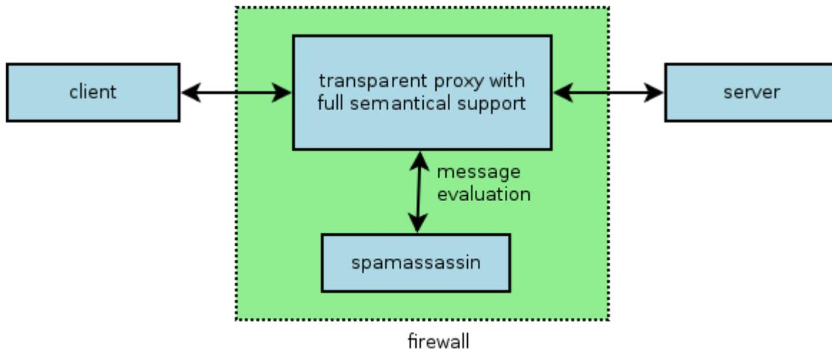
*Illustration 1: IMAP-filtering architecture with application level proxy*
